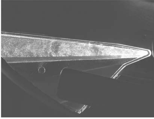
Fig. 2 Converging PIV light sheet with thickness tailoring.
