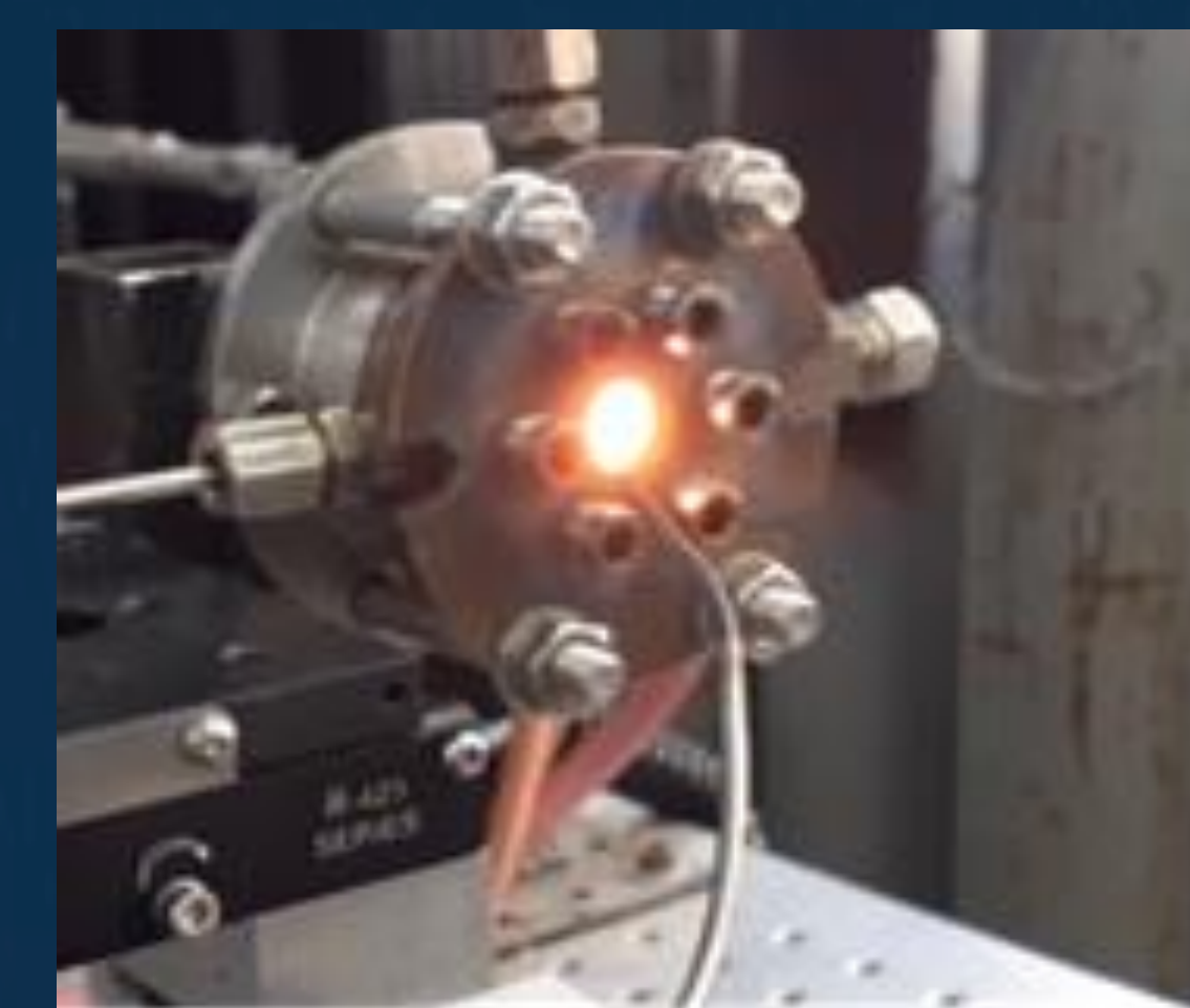
Proof-of-concept combustor in a test rig (left). The same combustor in operation (right)
