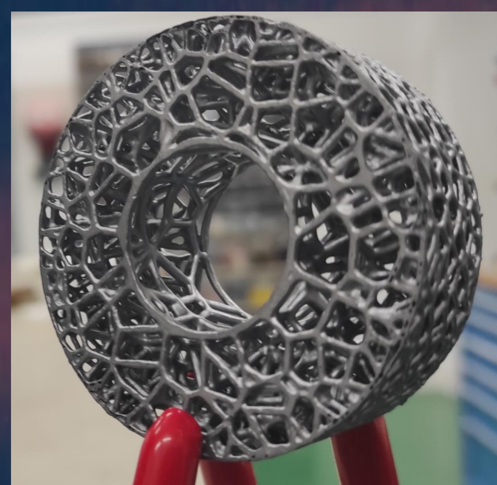
Two porous foams from Silicon Carbide
