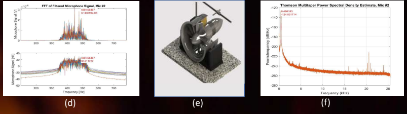
BOTTOM LEFT: Amplitude plot of microphone signal acquired downstream with one stator (shift in peak frequency is observed)
