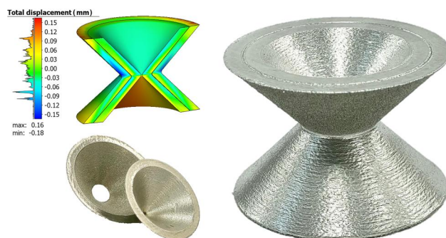
Fig. 17 Precompensation and manufacturing method validation by 45\text{ deg} double cone geometry with 300\text{ }\mu\text{m} clearance
