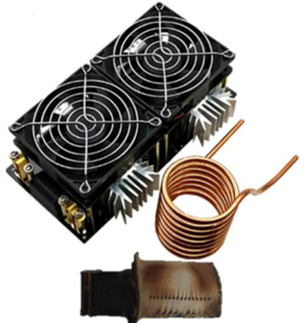
Fig. 4 Induction heating circuit and TBC coated turbine blade
